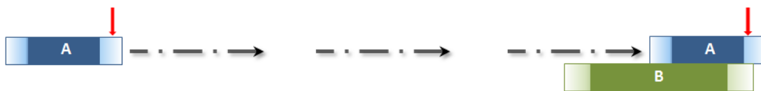
Figure 20: Temporal entity A ends before or with the end of temporal entity B. Here A is shorter than B
